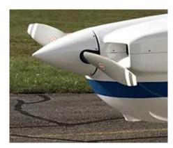
This new TB aircrafts spinner is entirely made of composite materials (carbon fiber combined with fiberglass) and is coated with a white gelcoat on the surface in standard.
