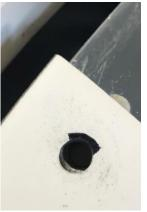
When the type of defect is met, the Ø5,1mm holes should be increase only in lateral direction:
