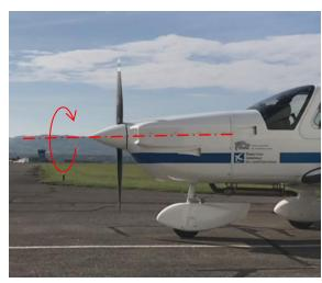
The static rotation test should be carried out over the entire rotation range of the engine. In the first time, make an evaluation during the engine rotation.
