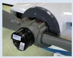
In previous mounting, adhesive tapes may be affixed on the back plate to reduce the clearance between it and the old aluminum spinner. With the new composite spinner, it is imperative to remove all adhesive tapes which are on the back plate or on the propeller because it can be create mounting defect. If necessary, restore the aluminum protection. Indeed, the adhesive tapes are sometime too sticky; it is possible the primary comes with it.
