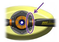
Once the desired pitch angle obtained, slightly tighten the **assembly screws of the hub**, those around the foot blade and then perform the same operation on each of the other blades.
