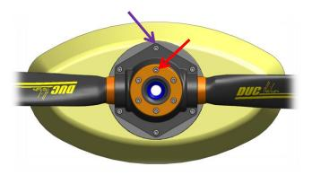
Slightly untighten the **propeller fixing screws** and the **M8 hub assembly screw**.
