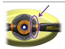
Once the desired pitch angle obtained, slightly tighten the M8 assembly screws of the hub, those around the foot blade and then perform the same operation on each of the other blades.
