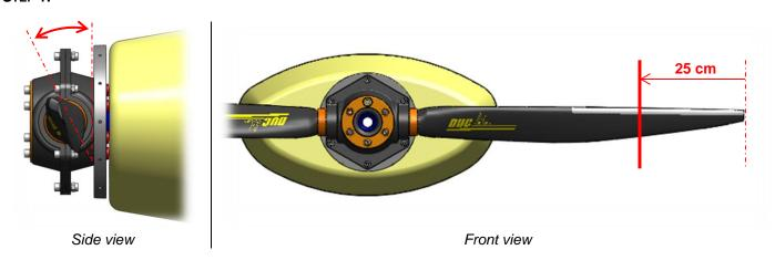
For the setting, the concerned blade must be placed in horizontal position.
