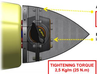
Assembly of the 2-blade, 3-blade & 4-blade hub:
