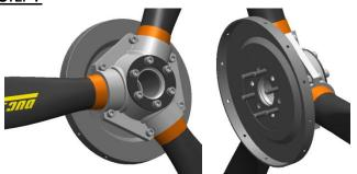
From the back, position the spinner mounting plate according the screws. Be careful to respect the direction of the plate. STEP 8
