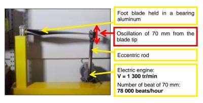
DUC blades suffered a bending test for 30 hours or 2 340 000 cycles of oscillation of 70 mm.
